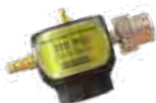
PRESET REGULATOR 215 PSI CGA (14.8 BAR) Piston Type 5,500-0 psi / 379.2-0 bar CGA 347/346 inlet Net Weight: 3.6lb 1.6kg Part No. 22-895401G3
